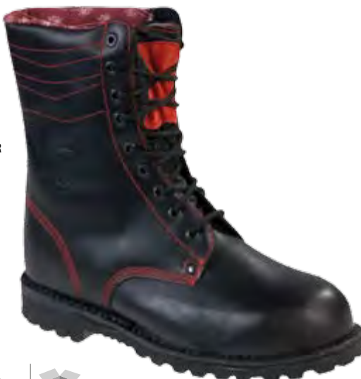
EN 345-1 S3 HI CI HRO EN 345-2 CLASS 2 PPE Cat II. Waterproof full grain greased heavy duty boots. Heat resistant (300°C) NBR rubber outsole "ROCCIA". Resistant to chain saw cutting.
